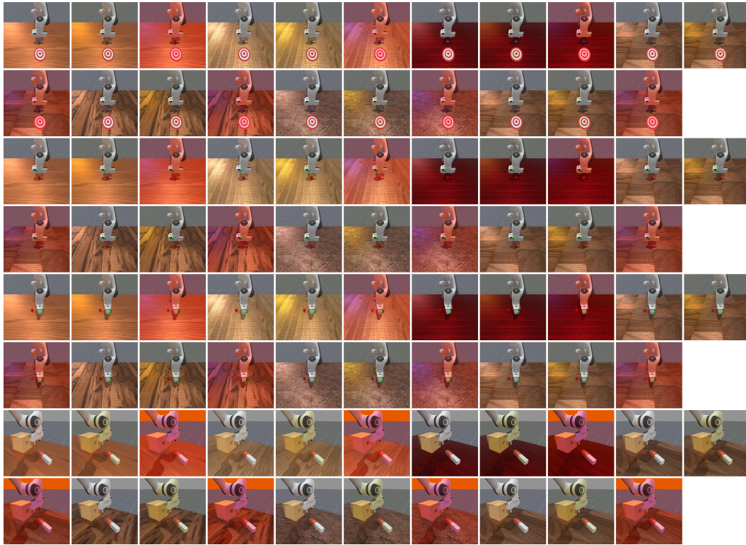
Figure 7: Sapien Testing Settings. Each task consists of 21 distinct settings, arranged in two rows. The images are grouped in threes, with each group sharing the same tablecloth texture but differing in lighting conditions: white, yellow, and red light. A total of seven unique tablecloth textures are used.
